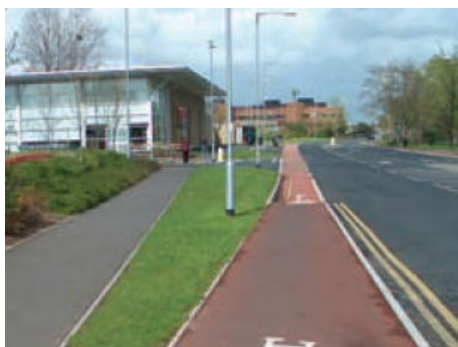
Reintroduction of the cycle path onto the carriageway, prior to a side road.
